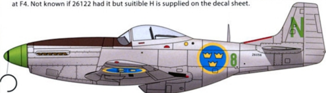
J 26, 26056, green Niklas F8 - Barkarby/Stockholm. The black walkways on the wings are of the last design, i.e. angled out towards the gun ports. The gun ports were also covered since these were liaison aircraft. This is the aircraft the general Nordensköld frequently used. The a/c earlier had an AN/APS-13 antenna.
