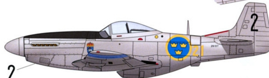
S 26, 26107, 2 - F21 Kallax/Luleå. Three blue stripes were painted on the wing tips, top and bottom. The size of the stripes was approximately 120 - 150 mm wide. The a/c had earlier been equipped with an AN/APS-13 antenna. Most likely the call sign was painted under the nose in standard fashion. It's hard to determine the size, later 800 mm was standard but as 26146 had 600 mm high numbers, this size may have been used under the nose of 26107.
