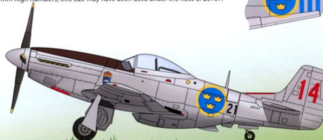
S 26, 26043, red 14 - F21. The last Mustang in the Swedish air force. Most likely dark brown anti-glare panel. Last design of walkways, i.e. angled toward the gun ports, see topside view, both port and starboard wing.
