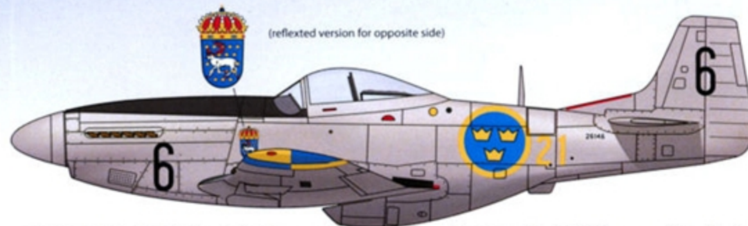
S 26, 26146, 6 - F21 Kallax/Luleå. Reconnaissance version of the J 26 with sKa10/50 camera in the fuselage. Call signs on both sides of the nose instead of underneath the nose which was standard. Blue and yellow fields on wing tips, top and bottom. The spinner was painted silver dope, just like the wings. The walkways on the wings were of the latest design, i.e. angled towards the gunports. Also note that all S 26 had their antenna mast moved forward and to right due to the camera installation. The anti-glare panel on the nose was black on some S 26.
