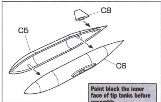
Paint black the inner face of tip tanks before assembly.
