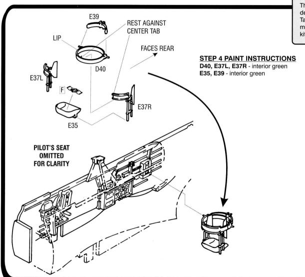
The components that make up the turret ring, seat and gun are delicate and molded in scale. They should be handled with care. Take your time and allow plenty of drying time. The rear gunner's machine gun is best assembled and installed toward the end of the kit construction to avoid breakage. (See Step 13)
