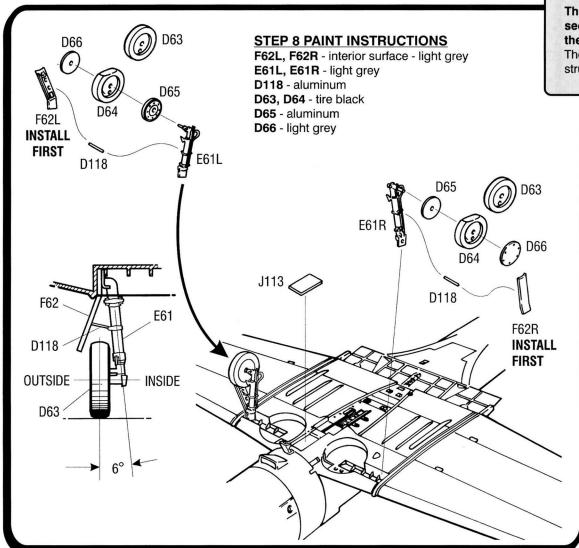
The landing gear assembly on this kit will "self align" if you follow this sequence of assembly. Difficulty with alignment can occur if you alter the sequence. (We told you it was a good idea to read these instructions!) The locating area in the wheel wells are designed to force the landing gear strut cover and the strut to have a precise relationship with each other.
