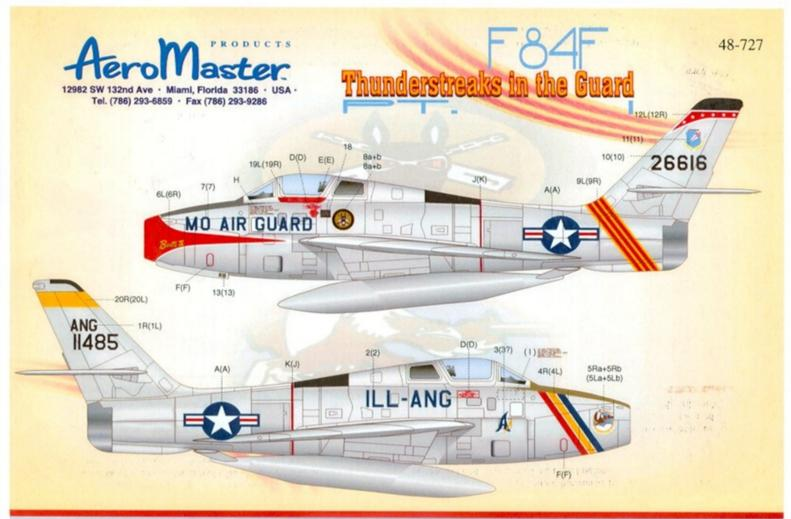
a/c 1- F-84F-40 RE, S/N 52-6616, 110 TFS/ 131 TFW, Missouri ANG. Squadron commander's A/C. Overall Natural Metal a/c with Black antiglare panel, fin tip and dorsal section. White wall on nose gear tire. We cannot read clearly the name of the pilot, but it looks like Major Pat Collins. It is shown on both sides of the cockpit, as it was favored in National Guard Units in those days.
