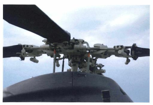
**NOTE** the arrangement of the rotor blade pitch control levers, and how they attach to the swash plate and the rotor head.
