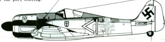
FW-190A-4, W Nr 581?, 1./JG1, 1943. Flown by Hpt Hans Khlers, *Gruppenkommandeur* of I./JG1. Factory camouflage of RLM 74/75/76. Cowling striped in black and white. Spinner RLM 70. Fuselage cross is white outline style with center in RLM 74. It is not known if the JG1 emblem was carried on both sides of the fuselage.
