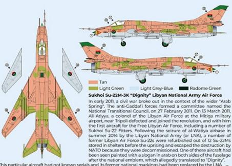
This particular aircraft had not known serials and its former national markings had been replaced by the LNA AF flag and roundels. Paint scheme consists of a worn out application of. Tan (FS 20450) and Light Green (FS 34128) over Light Grey-Blue (FS 36495). Nose cone, tail tip and dorsal antennas painted in Soviet Radome Green (FS 14090).
