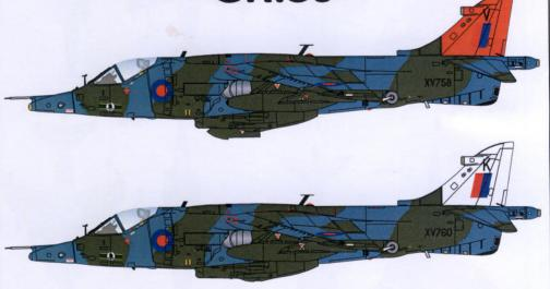
For the best results these decals should be applied to a gloss surface such as provided by either Xtracolor or Xtracrylix paints. Cut out the decal required and soak in warm water until the decal is released from the backing paper. Wet the area to be decaled with MICRO SET which will help to eliminate air trapped under the decal and position the decal.
