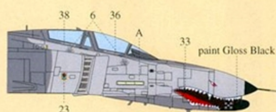
F-4G of the 561 FS/57 FW. Sharkmouthed F-4G Phantom (69-7295) (below & left), also of the 561FS/57FW, again Dark Gray FS36118 over Medium Gray FS36270. This machine was painted to commemorate the F-4 family's 33-year USAF service. Paint the forward nose pod Gloss Black before applying decals 32 and 33.
