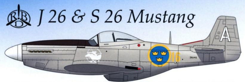
J26, 26046, white Alpha (Adam in SwAF) (later red A with the same badge) F16 Uppsala. Note that the antiglare area continued up and around the windshield frame. Walkway on left wing only. Also note the low placement of the serial number and red fuel caps just like the rest of the first fifty delivered
