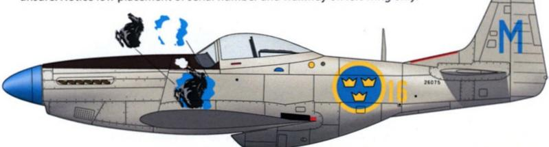
J 26, 26075, blue Mike (Martin in SweAF), second squadron F16 Uppsala. Propeller without cuffs (the thick part at the blade rot). Most likely walkway on left wing only. Detached AN/APS-13 antenna on vertical stabilizer (this left a little panel that a/c without the antenna didn't have). The horse badge is separated in two parts to make it possible to use with a/c that did not have the
