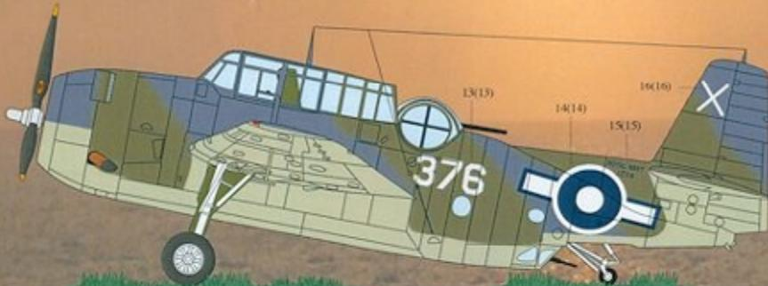
Avenger I, 711 Sqd, 1945. Sides and lower surfaces are White. Upper wings, tailplane and top of fuselage are camouflaged in Extra Dk. Sea Gray/Dk. Slate Gray. Leading edges of wing (1/4 chord line) and upper nose are black (night). A/C used for anti UBoat and Minelaying operations. Codes are Yellow on Blue panel.
