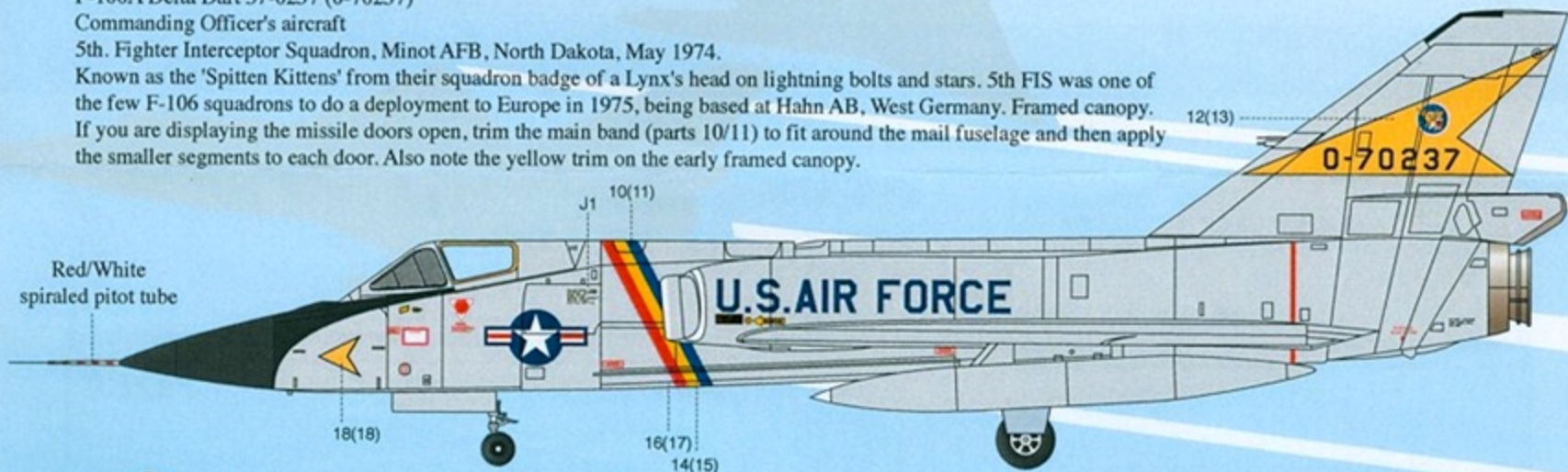
F-106A Delta Dart General plan view of upper surfaces indicating positions of insignia and stencils.
