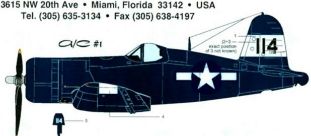
F4U-1D of VMF-214 or -216, USS Wasp (CV-18), Feb. 1945 during the first strikes on Tokyo. Overall Glossy Sea Blue, Propellers were Black with Yellow tips. Note position of individual aircraft number on a gear door. Natural metal prop Hub.
