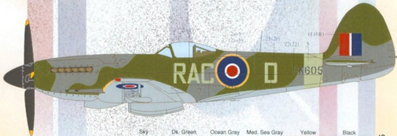
Spitfire F.22 PK605 502 Squadron, Royal Auxiliary Air Force, 1948. RAF Dark Green, Ocean Gray and Medium Sea Gray camouflage with Black spinner. Photo's suggest that, with service wear, the finish was semi-matt.
