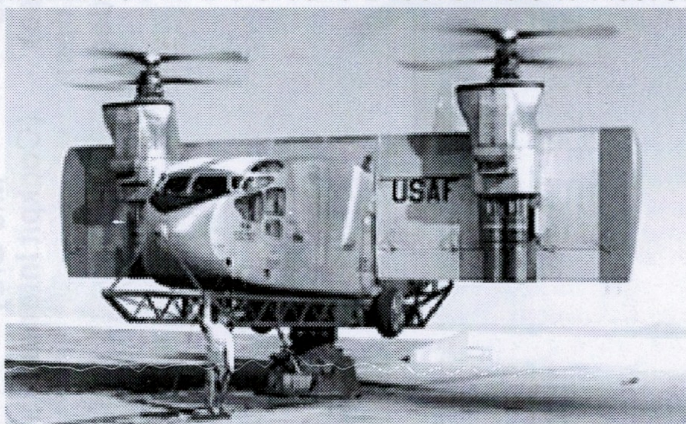
The X-18 was tested on the Ground Effect Simulation test stand
