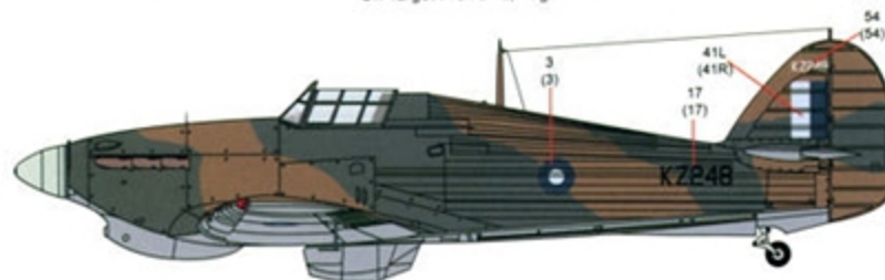
Hawker Hurricane Mk.IV, serial KZ248, of 28 Squadron, RAF, based at Kuala Lumpur, Malaya, late 1946 Pattern SEAC Day Fighter Scheme of Dark Green and Dark Earth over Medium Sea Grey undersides. Sky Type S Spinner. On-Target Profile 12, Page No 46
