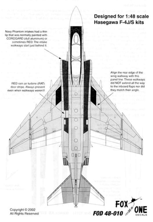
This decal set was designed to give the modeler maximum versatility for applying walkways for up to nine Phantom models. It provides the most commonly used walkway styles on U.S.Navy Gull Gray/White and some overall Gull Gray schemes. The walkways were drawn using factory drawings and adjusted to fit the 1:48 scale Hasegawa F-4J/S models. They do not fit the Hasegawa F-4B/N kits, which are completely different molds, or any other manufacturers' Phantom kits.
