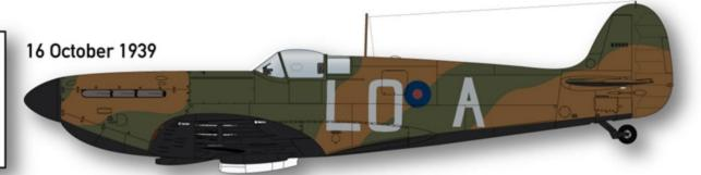
No. 602 Squadron's codes at this time were "ZT". The original Type A1 roundels have had their two outermost bands overpainted, and the white area overpainted with Ident Blue. This leaves us with a Type B fuselage roundel of the correct as-specified 15"
