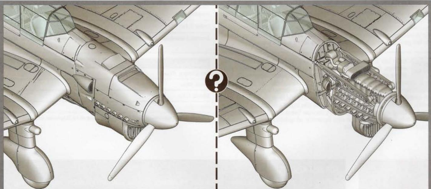
To build the model with the engine cowlings in place miss out steps 34 to 52.
