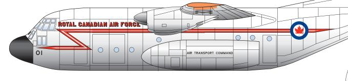
RCAF Hercules carried high visibility markings on wings and tail surfaces (above and below). On the earliest variants, these were fluorescent red-orange. Wing panels were 60"x 144", lined up with the leading edges as shown. On the wingtops, 84" RCAF roundels were centered 42" inboard of the aileron inner edge. Under the starboard wing was RCAF in 48" black letters; under the port wing, the last 3 of the serial.
