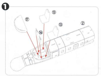
Paint the cockpit grey FS 36231. The inner frames are light tan. The controls (parts #14) and dashboard (part #17) are matt black. Use decal #50 for the instrument panel and attach it inside the cockpit. The seats (parts #13) are blue.
