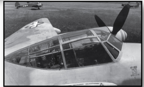
View showing the flat-sided main canopy on a B.Mk.VII. This canopy style was unique to Canadian built aircraft
