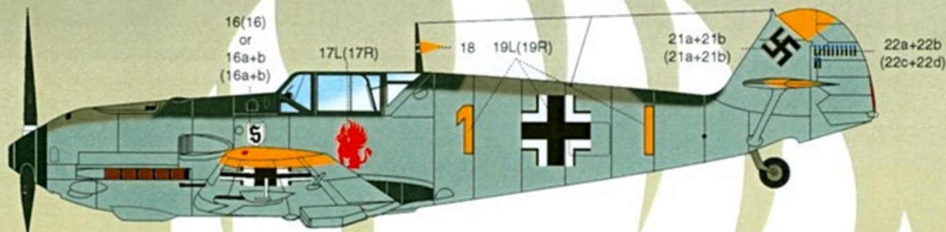
Bf-109E-4 flown by Oblt. Gerhardt Schöpfel, Staffelkapitän 9./JG26, August 1940, France. Camouflage is RLM 71 Dunkelgrün and RLM 02 Grau uppersurfaces, RLM 65 Hellblau undersurfaces and RLM 70 spinner. Note the RLM 04 Gelb Tactical Identification markings on wingtips, horizontal tail surfaces, and rudder.
