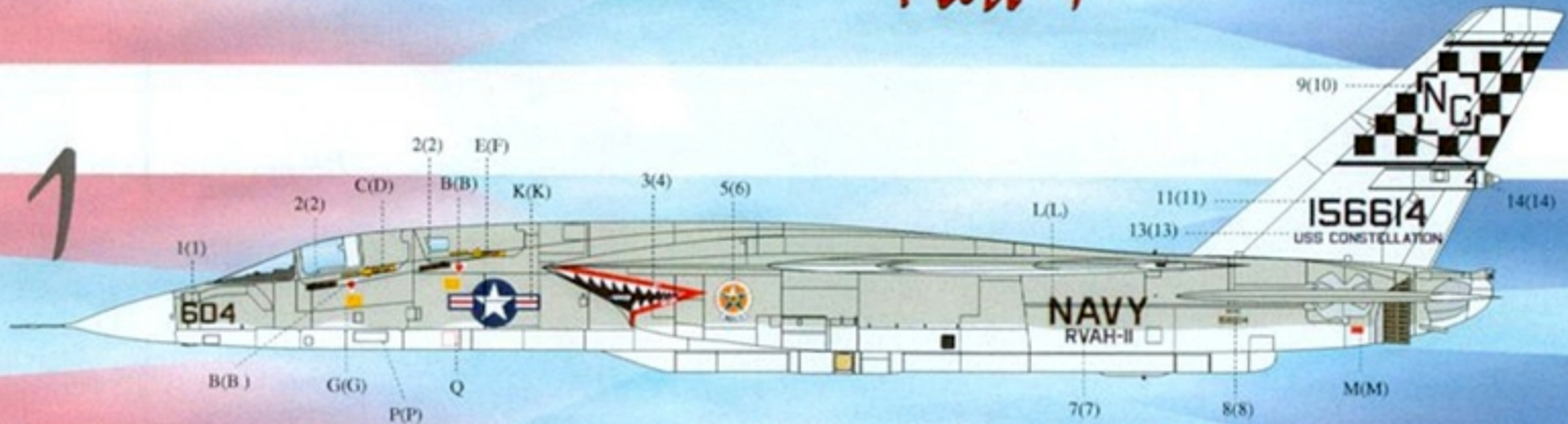
RA-5C Vigilante BuNo. 156614. The Checkertails of RVAH-11 were aboard USS Constellation (CVA64) during the Linebacker operations in the Spring of 1972. Non-specular Gull Gray FS36440 upper surfaces with Gloss White FS17875 vertical tail, undersides, control surfaces, radome, landing gear, and wheel wells. Wing leading edge slats Dark Gull Gray FS35231; edges of gear doors painted FS11136 Insignia Red.
