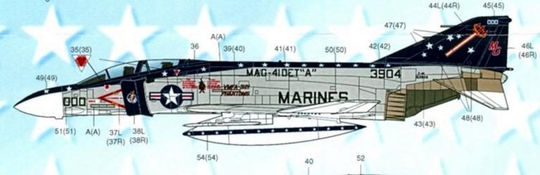
A/C 2 • F-4S Bu No153904 VMFA-321. Same colors as A/C 1 with the following differences. Complete spine, vertical fin and rudder, antiglare panel and intake ramp are Gloss Insignia Blue. Upper surface of flaps is also Lt. Gull Gray.
