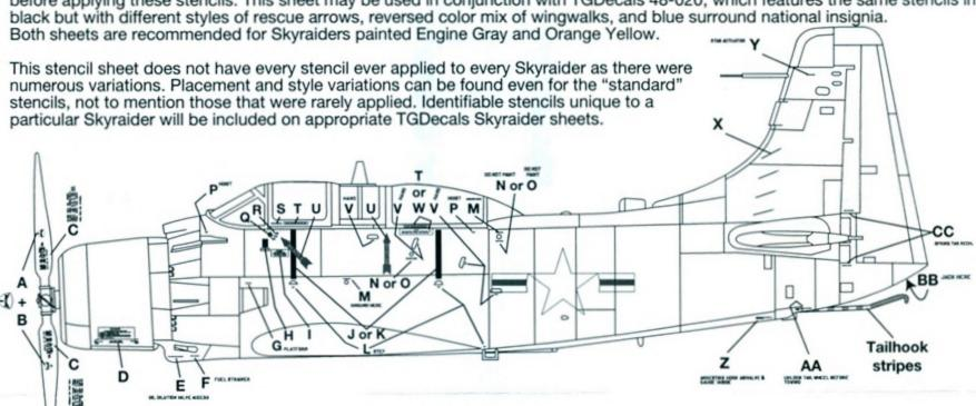
The Aeroprop logo (A+B) points to the left when a propeller blade that is pointing upward is viewed from the front.
