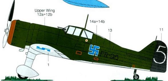
Finnish Air Force D.XXI, FR-96 of Lentorykmentti 2 (Air Wing 2) during the Winter War, 1940. Dark Olive Green/Gray Scheme. Black rudder. Note that the propeller blades are Aluminum — with only a portion of the backs in anti-glare Back. Note, too, the "toned-down" national markings on all upper surfaces, with regulation blue/white national insignia beneath the wings.
