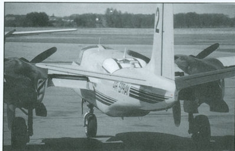
Note beacon locations on #2 and #12 are different.
