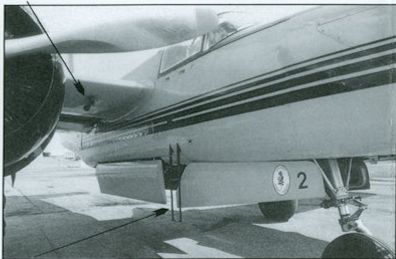
#2 has a fixed ladder that does not retract into fuselage.
