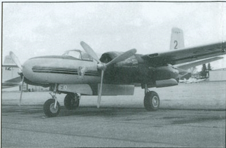
Note venturi on right wing. Same location for #12.
