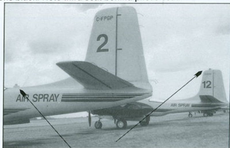
Note beacon locations on #2 and #12 are different.
