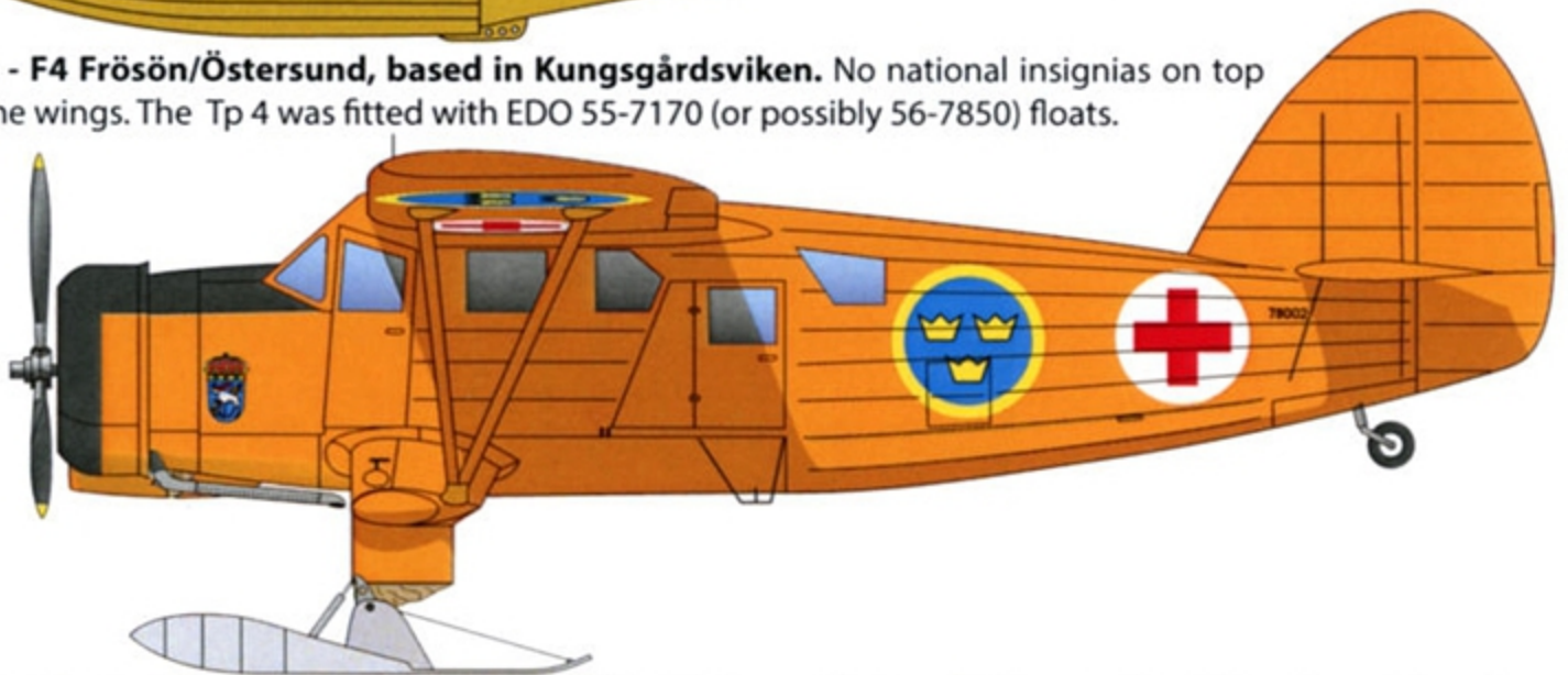
Tp 78, 78002, c/n 601 (USAF 44-70336) F4 - Frösön/Östersund. Three blade propeller, skies painted silver dope (same model as ASJA B 5 etc). Exhaust pipe with cabin heating and airframe painted in Swedish Air Force Orange (close FS 22243). This a/c was probably fitted with EDO 55-7170 and the curved attachments struts during the summer. The a/c was back at F2 1954-06-29 but crashed 1954-07-14 at Blidö.
