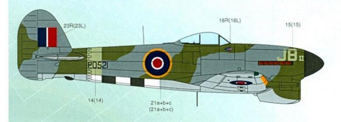
JB II, Serial No. PD521, Typhoon Mk IB of No. 146 Wing. Flown by Wg Cdr J. R. Baldwin. B.70 Antwerp, November 1944. Camouflaged in Ocean Gray and Dark Green over Medium Sea Gray. Sky fuselage band. Black spinner. Invasion stripes on fuselage bottom only. Tempest tail plane on this A/C. Four bladed prop.
