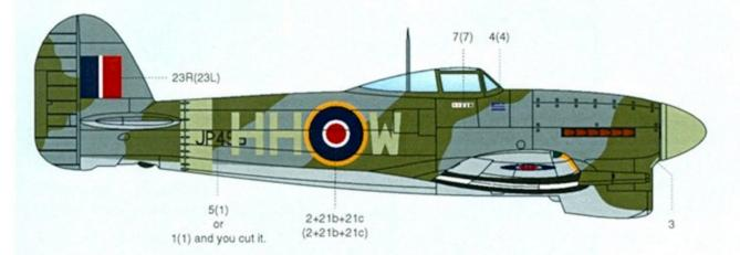
HH•W, Serial No. JP496, Typhoon Mk IB of No. 175 Sqn. Flown by Sqn Ldr R. T. P. Davidson. Lydd, September 1943. Camouflaged in Ocean Gray and Dark Green over Medium Sea Gray. Sky fuselage band and spinner. I.D. stripes under wings. Left side codes read HH•W. Three bladed prop.
