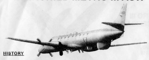
The Fairchild (Swearingen) Metro have been one of the most sold commuter aircraft in the class up to 20 seats. The aircraft had the advantage to be faster than many of its competitors and to be one of the first designs in its class with pressurized cabin. The large rear door made the aircraft also well suited for cargo operators.
