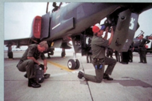
USAF ground crewmen service the KS-87 camera in an RF-4C. (below)
