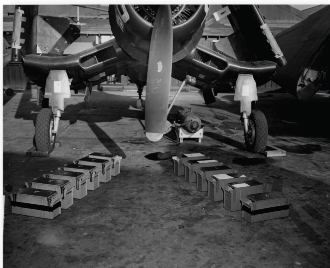
The above picture shows the color scheme developed by this Command for easily identifying ammunition cans during rearming with spare cans. The No. 3 cans are left the same color, green, as they come from the factory. The No. 4 cans are also green, except for a 2" black stripe all the way around. The No. 1 cans are painted red and the No. 2 cans are red with a 2" black stripe all the way around. The picture also shows parts of the white insignia (painted on the top of the left wing) on the tops of the No. 1 cans. This presents a serious problem in rearming and can be remedied by using the fuselage insignia on the top of the port wing and moving it 20" toward the wingtip.
