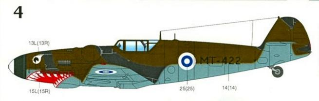
Bf-109G-6, MT-422, Finnish Air Force, HLeLv 31, Utti, 1948. Olive green (F.S. 34096) and black upper surface camouflage, lower surfaces It. blue grey (F.S. 35414). Spinner front white, RLM 70 back. Prop blades 70 with yellow tips.
