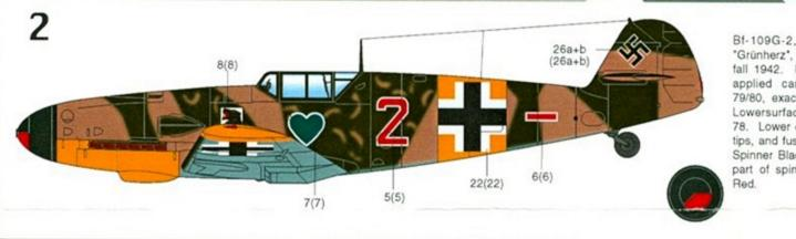
BI-109G-2, II./JG 54 "Grünherz", Siwerskaja, Russia, fall 1942. Non- standard field applied camouflage of RLM 79/80, exact pattern unknown. Lowersurfaces probably RLM 78. Lower cowling, lower wing tips, and fuselage band Yellow. Spinner Black (or possibly 70), part of spinner frontal area is Red.
