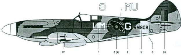
Spitfire F Mk XIVe, RM908, 152 Sqdn, RAF, 1945. Dark Green, Ocean Grey and Medium Sea Grey camouflage with white spinner. Codes read "UM-G" on port side of fuselage. White SEAC theatre bands (24") on upper and lower wings and tail surfaces. Note squadron codes partially cover serial on port side.
