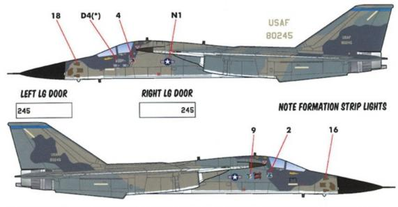
NOTE THAT CONFORMAL ANTENNAS ON THE NOSE ARE VISIBLE ON THIS JET - USE DECALS 16 AND 18 AS SHOWN
