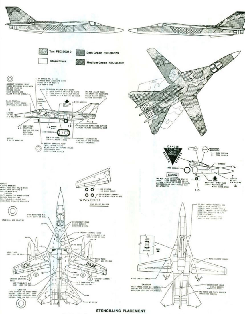
Stencilling data given on this sheet is basic. For complete stencilling data refer to decal sheet 48-229.
