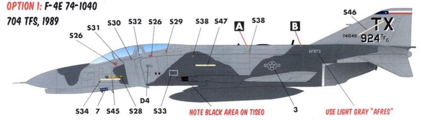
74-1040 WAS ONE OF THE F-4E PHANTOMS OF THE 704 TFS PAINTED IN THIS SCHEME FOR THE GUNSMOKE '89 COMPETITION AT NELLIS. NOTE THAT THE AIRCRAFT IS EQUIPPED WITH TISEO AND AN/ARN-101 ANTENNA ON THE SPINE.
