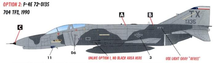
MAINTENANCE STENCILLING IS IDENTICAL TO THAT OF OPTION 1. LIKE MOST OF THE UNITS F-4E'S, THIS AIRCRAFT IS ALSO EQUIPPED WITH TISEO AND AN/ARN-101.
