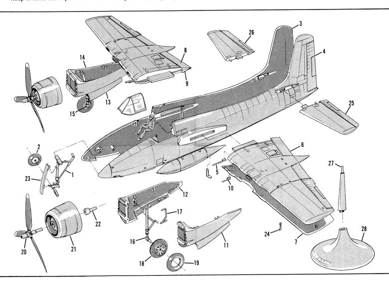
Slip nosewheel 2 onto axle portion of front strut 1 and flare over end of axle with the heated blade of an old knife. Cement pins on strut into holes in right fuselage half 3. Cement hole in pilot's back onto pin in rear of cockpit on fuselage half 4. Cement fuselage halves 3 and 4 together. Cement stabilizers 25 and 26 into slots in rear of fuselage. Check stabilizer to make sure it is straight while cement is drying.
