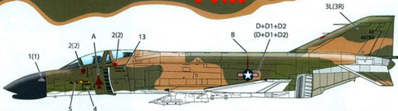
F-4C-23-MC Phantom II 64-0752. Flown by Maj Paul Gilmore and 1/Lt. William Smith of the 480th TFS, 35th TFW, Da Nang, South Viet Nam, when they downed a MiG-21 with an AIM-9B on 26 April 1966. T.O. 1-1-4 camouflage. Radome and nose IR sensor Flat Black. Straight US Navy style inboard pylons and no tail ECM fairing. MiG-21 silhouette carried on the left inlet ramp.
