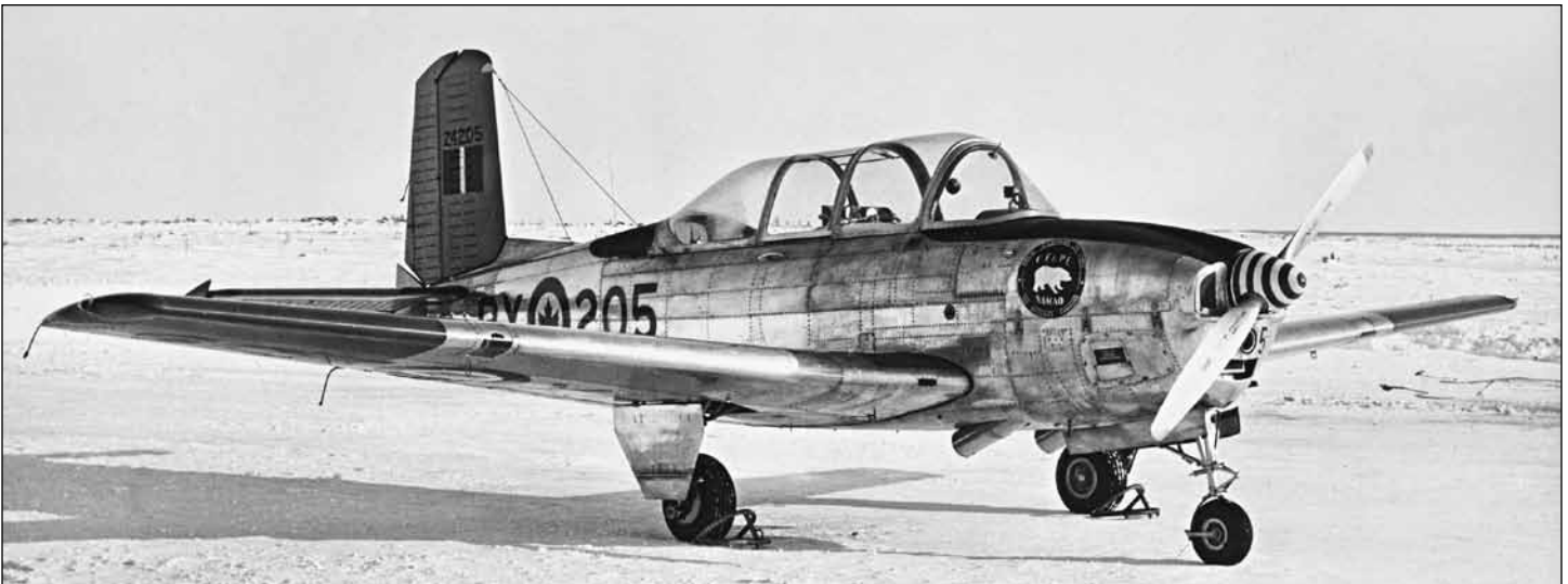
A winter view of Mentor 24205 at CEPE, but at what appears to be a later time than the first photo. For some reason the nose side number '205' is not present on this side of the aircraft. Also note that, just to the left of the prop spinner, there now appears to be an airflow restrictor over the normal radiator upper openings in the cowling. Changes to the colour scheme include the addition of the CEPE badge, CEPE's 'PX' codes to the fuselage and lower wings, the red/white ringed prop spinner. The red-painted wingtips are now clearly visible in this image; this addition of red 'search' markings on the wing tips and horizontal tailplanes was stipulated for aircraft being used on winter trials. Careful examination of the two CEPE photos will reveal that '205 had a propeller change during its time with the unit, resulting in two different prop tip markings. Here they are, having reverted to the conventional 4" yellow tips, compared to the more colourful tips that were first applied. Credit: the Ian Macdonald collection via the CAHS
