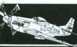
Cripes Third after the 29 June 1944 mission. Note the Invasion Stripes on top of the wing, the air breather plate, and the absence of the ground crew names forward of the wing root.
