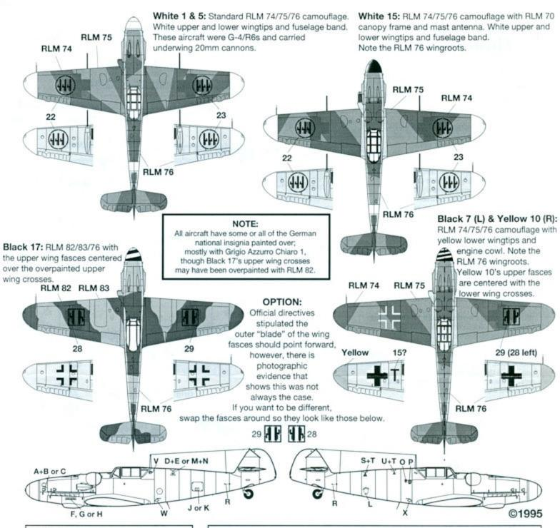
NOTE: Stencil markings, where known, have been called out on the individual side views of each aircraft. A set of Bf 109 stencils has been included and general placement is as shown above.
