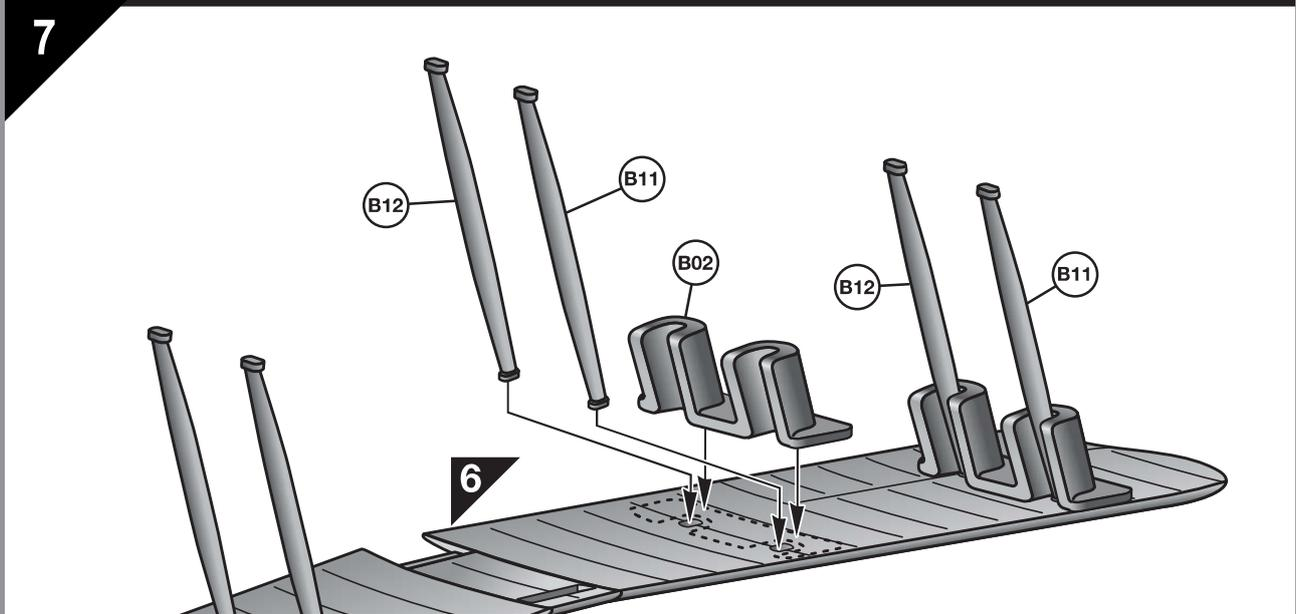
Parts B01 & B02 are not parts of the completed model. They are intended to help set the correct angle of the wing struts B11 & B12. Use cement sparingly so that B01 and B02 do not become fixed to the model.
