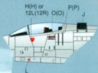
North American F-100D Super Sabre Plan view of upper surfaces showing general positioning of insignia and stencils.
