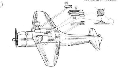
Cement the fuselage onto the wing and bombs in place.
