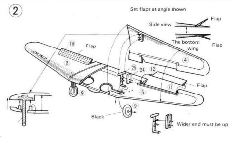
Place flaps  $\widehat{10}$   $\widehat{11}$  on  $\widehat{5}$ . Cement cover  $\widehat{24}$  to wheel leg  $\widehat{25}$  (2) and place on  $\widehat{5}$ . Do not cement these parts. Cement wing tops  $\widehat{3}$  and  $\widehat{4}$  to the lower wing and cement wheels to  $\widehat{25}$ .
