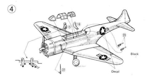
Cement pilot, gunner and machine guns as shown. Cement canopy sections and antenna in place. Apply decals.
